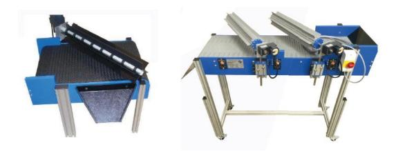
Plastic part sprue separation - plastic part runner conveyors with Paddle Separators are available in variable lengths and in a variety of widths and colours individually designed to meet application and space requirements.
